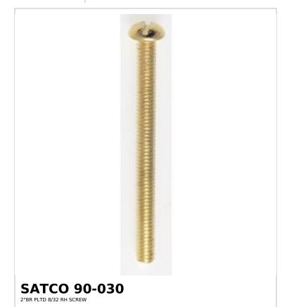
General Status Active Length (in.) 2 Finish Brass Plated 045923900303 Each UPC Physical Finish Family Brass Thread 8/32 Thread Screw Type Slotted Machine Round Head Material Steel Compliance
