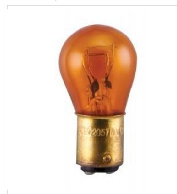
General Status Active Watts 26.88W/8.26W 12.8V/14V Volts Shape S8 Filament C-6 Base **Bayonet Double Contact** ANSI Base BA15d Finish Amber Hours Rated 1200 Product Category Miniature Technology Incandescent Electrical Amps 2.100/0.590A Dimmable Non-Dimmable Physical MOD 1 None Housing Color Compliance California Status Lawful for sale in California Title 20 / 24 Status Lawful for sale California Prop 65 Lead Colorado Status Lawful for sale Hawaii Status Lawful for sale
