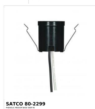
General Status Active Voltage 250V Wattage 660W Length (in.) 1.25 1.25 Width (in.) Height (in.) 1.5 Finish Black cULus - Listed Safety Listing Electrical Wire Color Black / White Wire Length 9 in. Physical 1.25 Diameter Extension (in.) 1.38 Finish Family Black Phenolic Plastic Material Additional Information 1-Year Warranty Compliance
