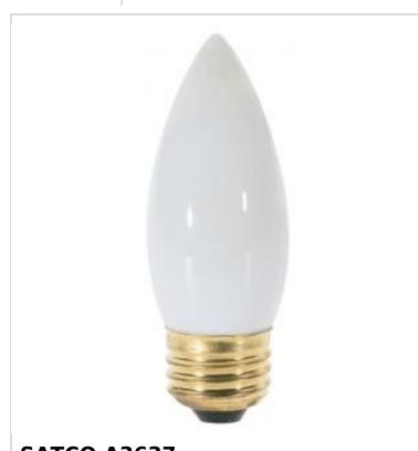
General Status Discontinued Watts 25W Volts 130V B11 Shape Lumens 160L Base Medium Filament CC-2V ANSI Base E26 Finish White CCT (Kelvin) 2700K Warm White Temperature CRI 100 Beam Spread 360 Hours Rated 2500 Product Category Candle Technology Incandescent Electrical Dimmable Yes-Dimmable **Operating Position** Universal Physical MOL 3.88 MOD 1.38 Compliance California Status Lawful for sale in California Title 20 / 24 Status Lawful for sale California Prop 65 Lead Colorado Status Lawful for sale
