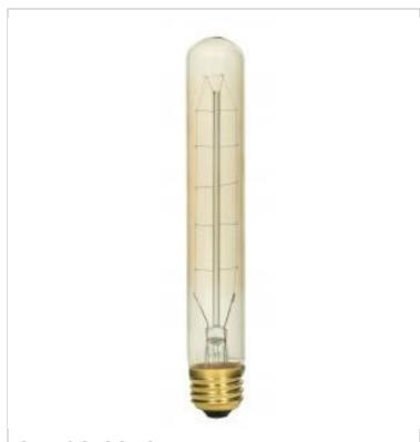
General Status Active Watts 40W Volts 120V Shape Т9 Filament Hairpin Base Medium ANSI Base E26 Finish Clear CCT (Kelvin) 2700K Temperature Warm White CRI 100 Lumens 160L Beam Spread 360 Dimmable Yes-Dimmable Hours Rated 3000 Product Category Tubular Technology Incandescent Physical MOL 7.31 MOD 1.09 Housing Color None Weight (lb.) 0.11
