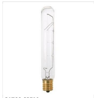
General Status Active Watts 40W Volts 130V Shape T6.5 Filament C-8 Base Intermediate ANSI Base E17 Finish Clear CCT (Kelvin) 2700K Temperature Warm White CRI 100 Lumens 350L Beam Spread 360 Dimmable Yes-Dimmable Hours Rated 1500 Product Category Tubular Technology Incandescent Physical MOL 5.38 MOD 0.81 Housing Color None Weight (lb.) 0.63
