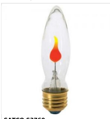
General Status Discontinued Watts 3W Volts 120V Shape CA9 Base Medium Filament Neon ANSI Base E26 Clear Finish 2700K CCT (Kelvin) Warm White Temperature CRI 100 360 Beam Spread 1000 Hours Rated Product Category Candle Technology Incandescent Electrical Dimmable Yes-Dimmable **Operating Position** Universal Physical MOL 4.56 MOD 1.13 Compliance California Status Lawful for sale in California Title 20 / 24 Status Lawful for sale California Prop 65 Lead Lawful for sale Colorado Status
