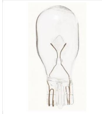
General Status Active Watts 10W Volts 24V Shape Т5 Base Mini Wedge ANSI Base W2.1x9.5d Finish Clear 126L Lumens Beam Spread 360 Hours Rated 2000 Product Category Miniature Technology Incandescent Electrical Amps 0.420A Dimmable Non-Dimmable Physical MOL 1.5 MOD 0.63 Housing Color None Compliance California Status Lawful for sale in California Title 20 / 24 Status Lawful for sale California Prop 65 Lead Colorado Status Lawful for sale Lawful for sale Hawaii Status Nevada Status Lawful for sale
